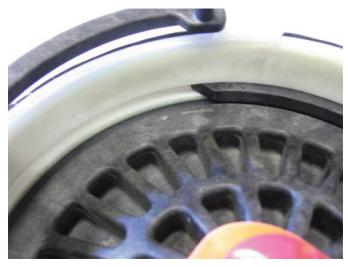
5. Install the angled lead tip of the retaining ring into the groove.
