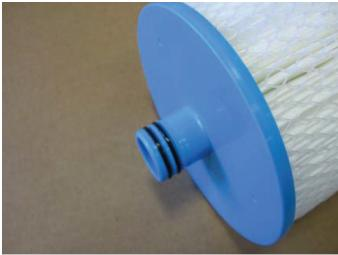
Ensure o-rings are properly lubricated before installation. Insert filter into the filter adapter of the bottom drain assembly.
