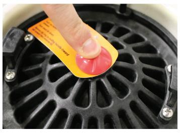
2. Remove top cover and relieve pressure in tank by pressing red button.
