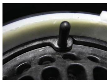
6. Working clockwise, push the retaining ring into the groove until the end snaps into place. Gently pull on lid assembly to seat o-ring.
