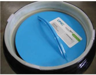
2. A filter this high is not installed properly.
