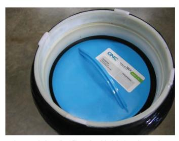
3. A properly installed filter should sit below the seal area.
